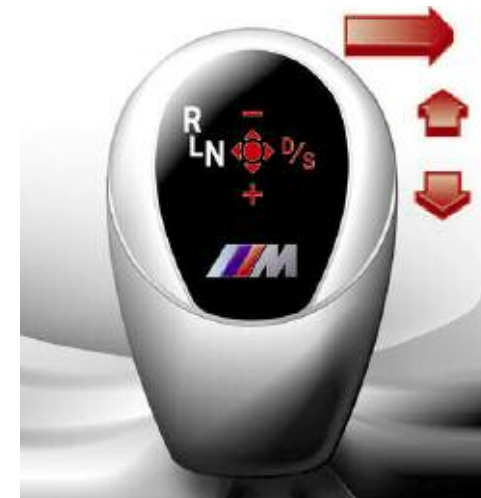
The M GWS pushed to the right twice to start sequential mode
